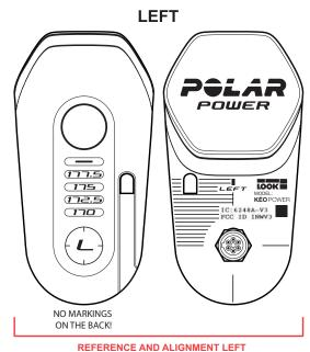
REFERENCE AND ALIGNMENT LEFT NOTE! MARKINGS SHOULD BE DONE BEFORE DIRT SEALING IS INSTALLED!
