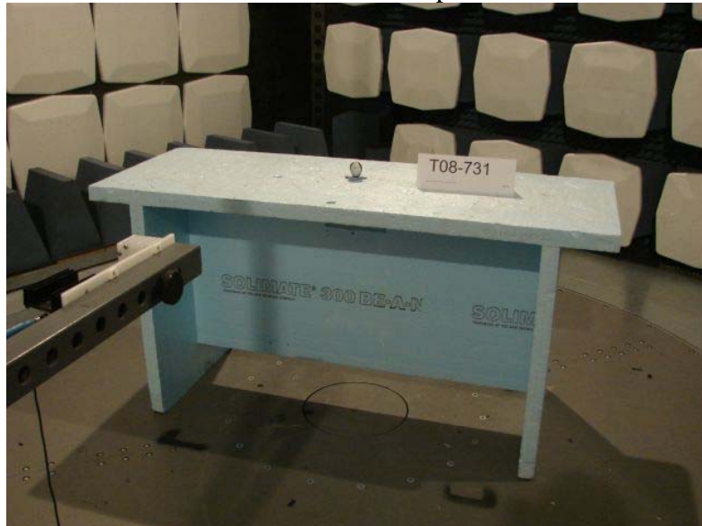
Picture 4: Radiated emission test setup 18 GHz – 25 GHz
