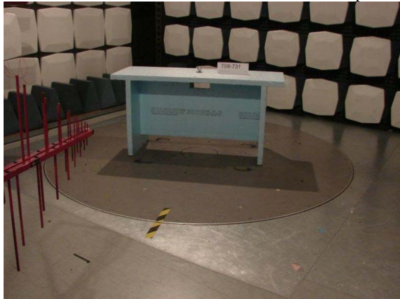
Picture 2: Radiated emission test setup <1 GHz
