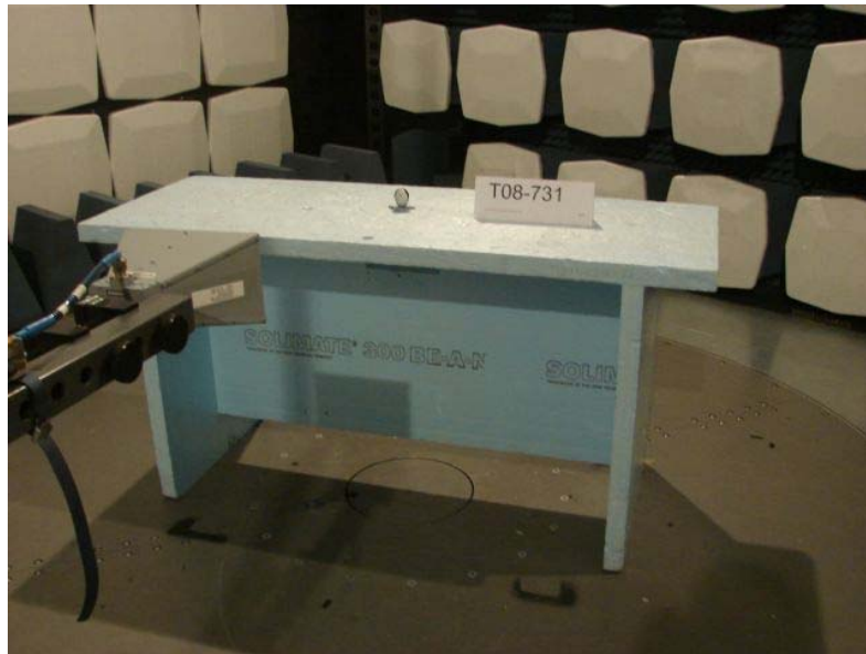
Picture 3: Radiated emission test setup 1 GHz – 18 GHz
