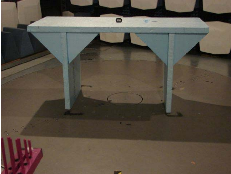
Picture 3: Radiated emission test setup <1GHz
