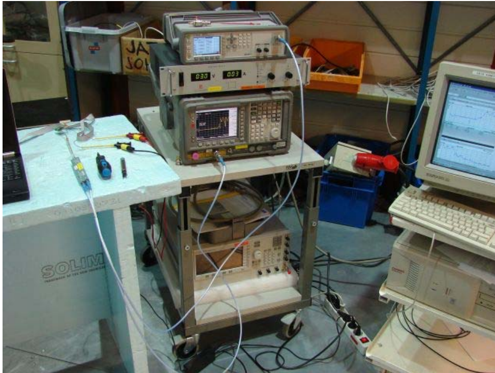
Picture 1: Conducted measurement test setup
