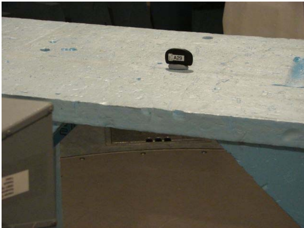
Picture 4: Radiated emission test setup 1 GHz – 18 GHz
