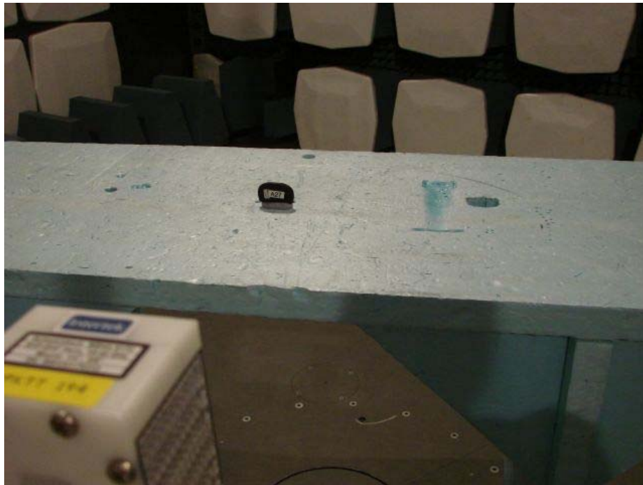
Picture 5: Radiated emission test setup 18 GHz – 25 GHz
