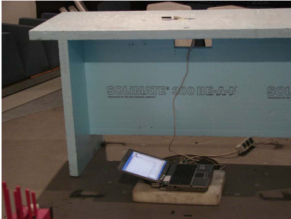
Picture 1: Spurious emission measurement setup
