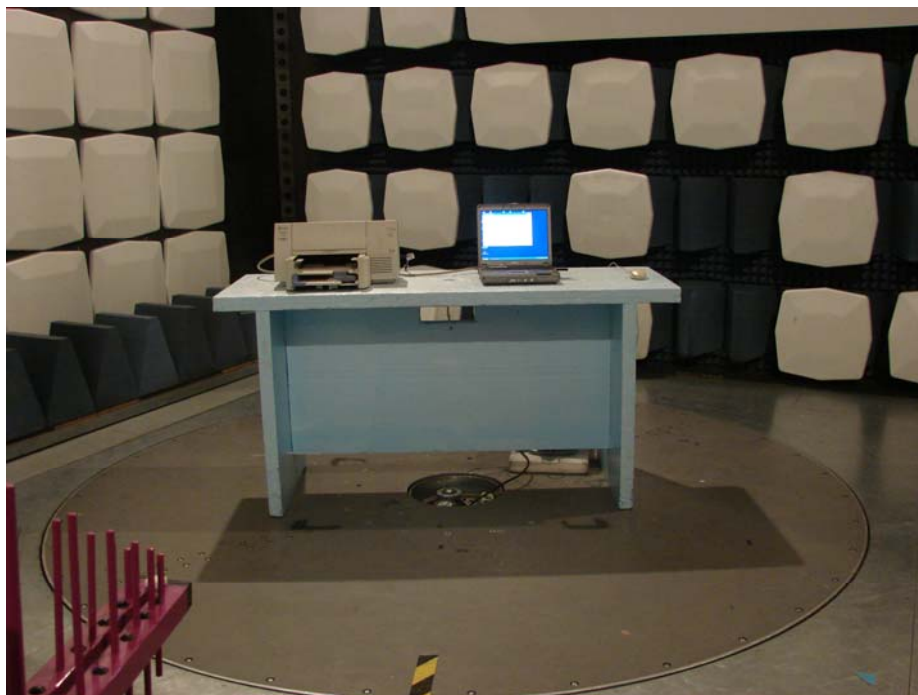
Picture 4 Radiated emission test setup
