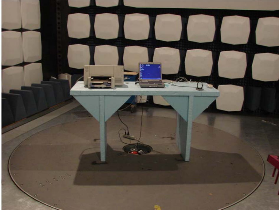
Picture 3: Radiated emission test setup
