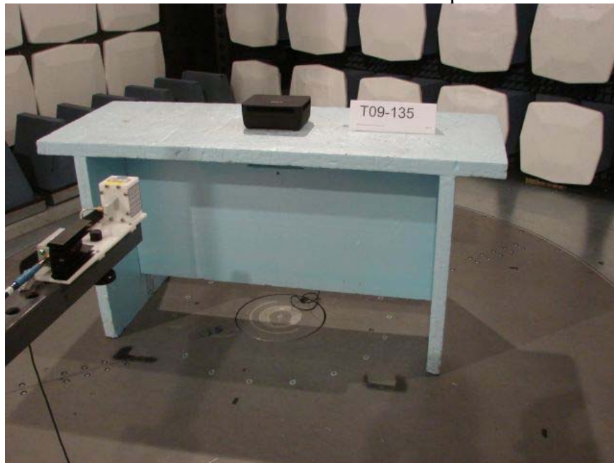
Picture 4: Transmitter Radiated emission test setup 18 GHz – 26 GHz.
