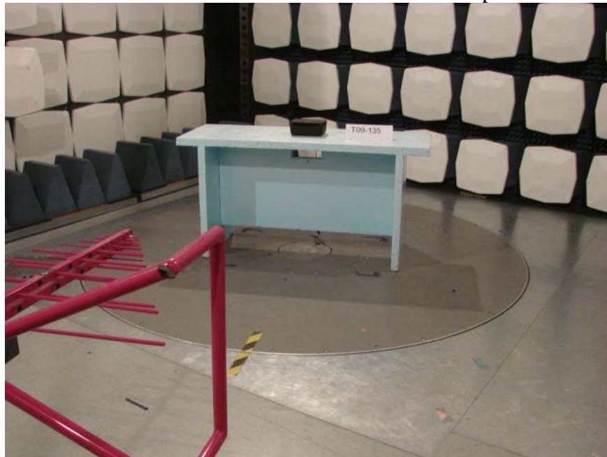
Picture 2: Transmitter Radiated emission test setup <3 GHz
