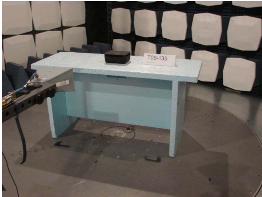
Picture 3: Transmitter Radiated emission test setup 3 GHz – 18 GHz.
