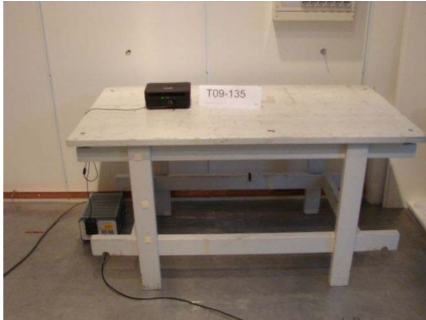
Picture 1: Conducted emission measurement test setup
