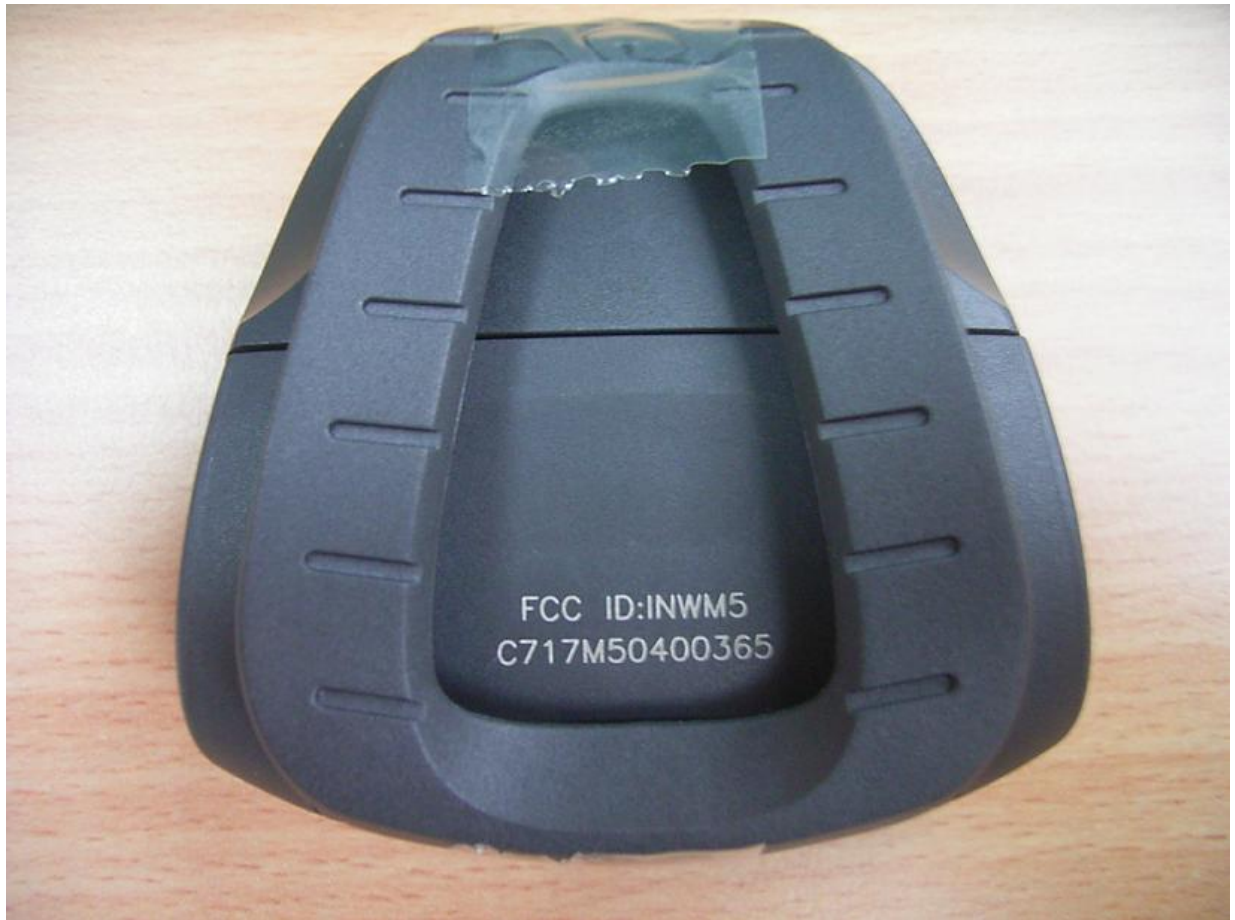
Picture 2, Final placing of FCC ID (cover closed)
