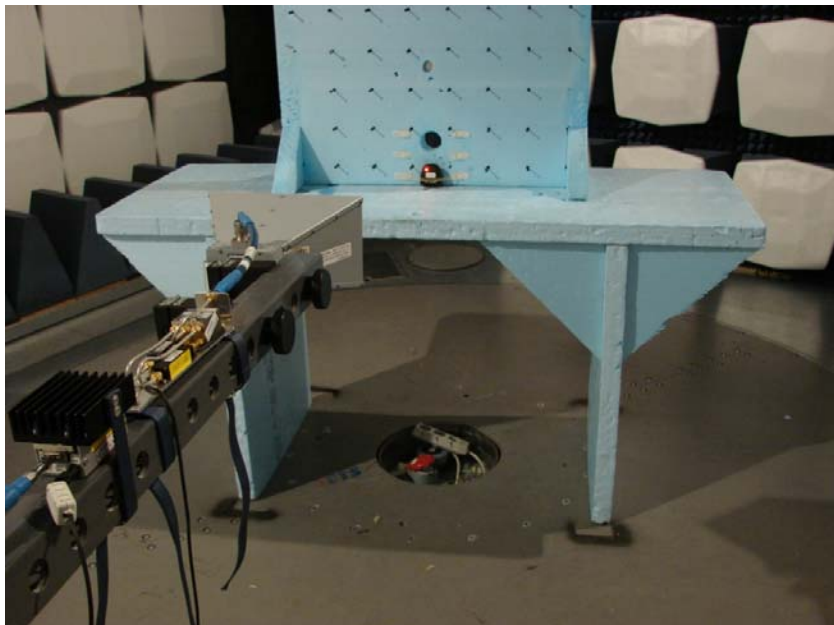
Picture 2: Spurious emission and field strength measurement setup
