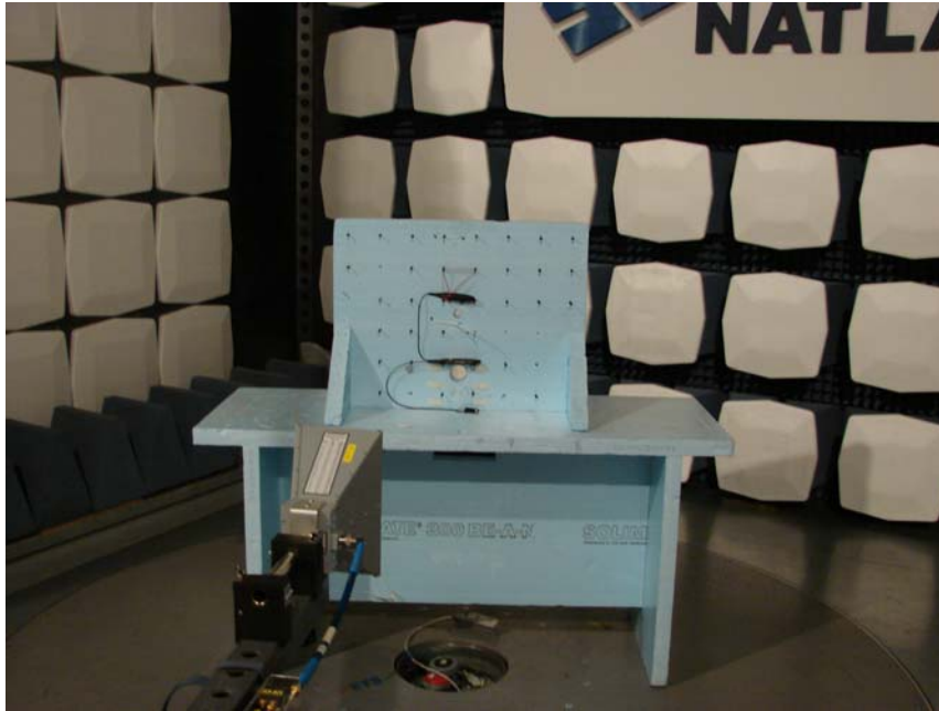
Picture 1: Spurious emission measurement setup
