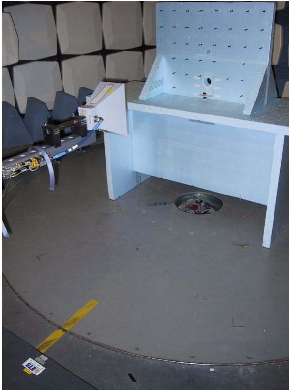
Picture 1: Spurious emission measurement setup
