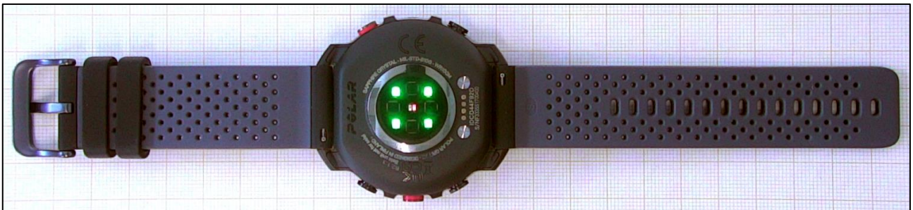
Figure 2. Device from behind, OHR and USB charging cable contacts are visible.
