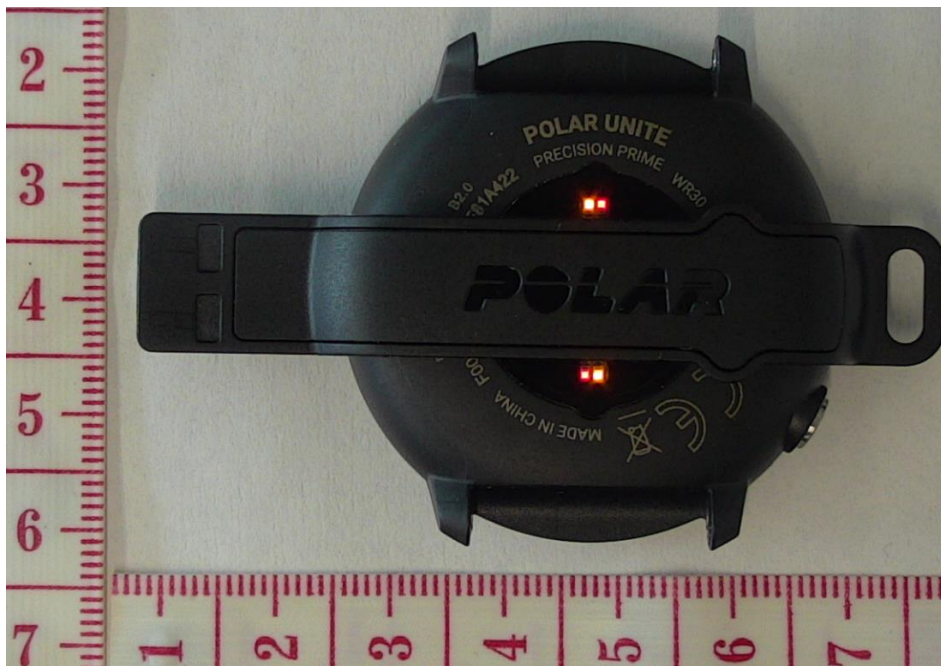
Figure 6. USB adapter inserted into the device.
