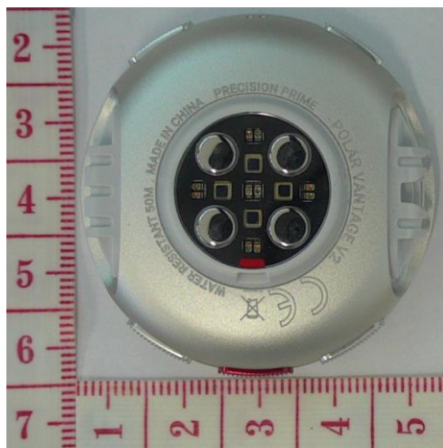
Figure 2. Device from behind, markings and USB adapter contacts are visible.
