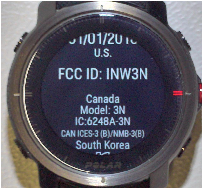
Figure 8. FCC ID and Canada ID markings.
