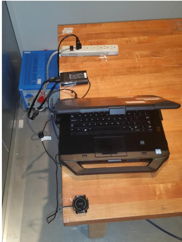
Figure B5. Conducted Emission Setup
