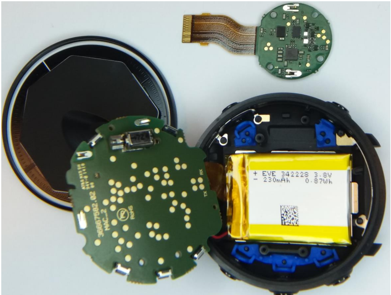
Figure 4. The OHR board is under the battery.
