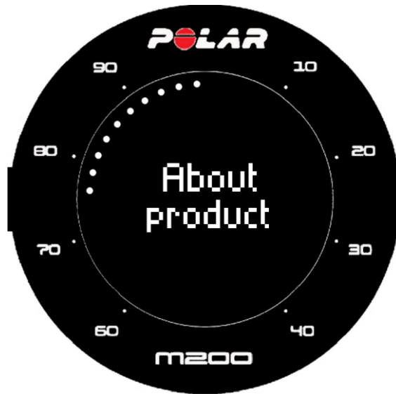
Figure 3. Press right button 3 times to get “About product” view and press with a long pressing to enter.
