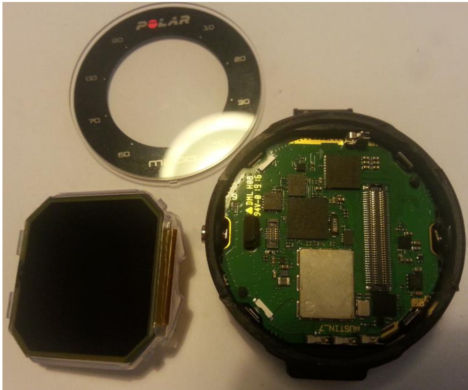
Figure 1. Lens and frame removed
