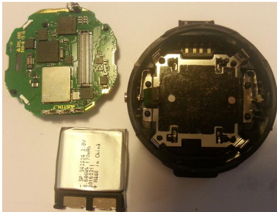
Figure 2. PWBA and battery removed
