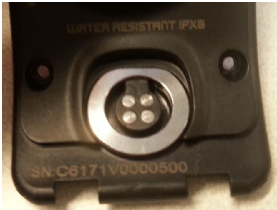
Figure 8. Module, back side (underneath), USB port
