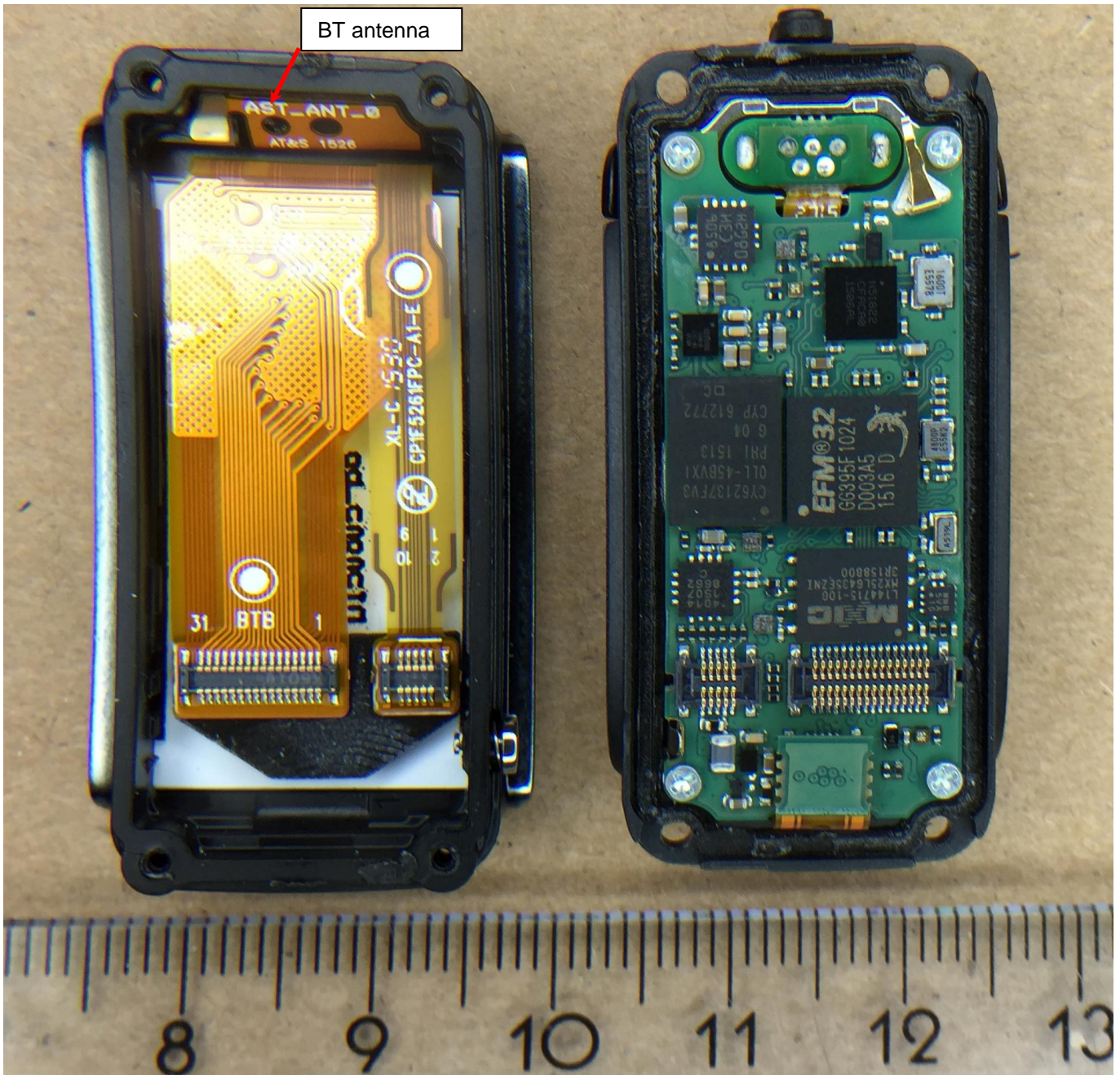
Figure 1. Display module and electronics module side by side.
