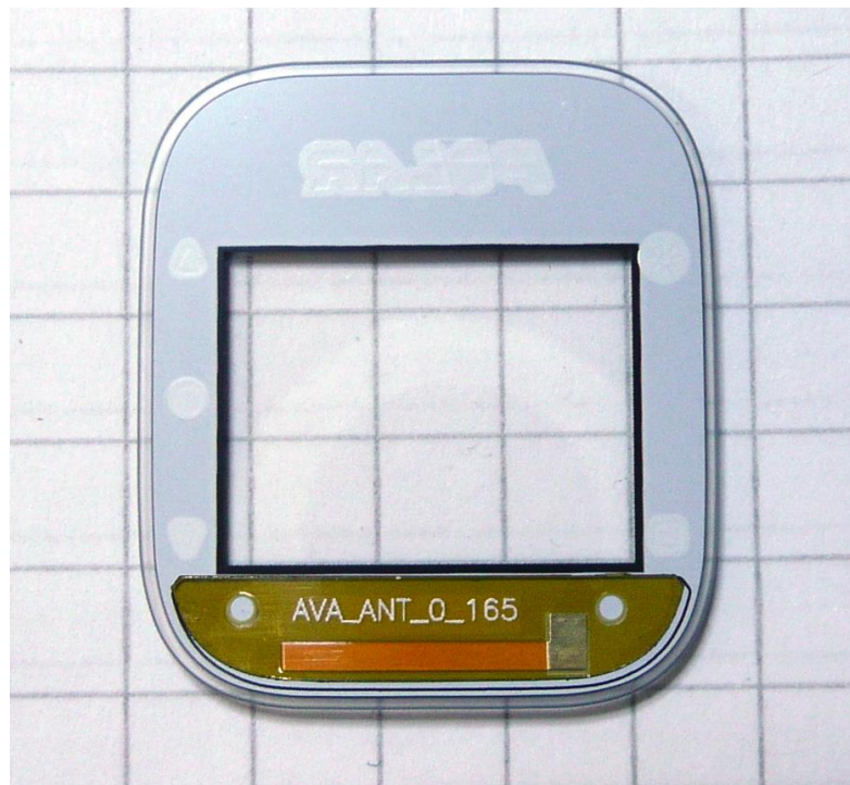
Figure 4. Back side of the lens assembly with the antenna.
