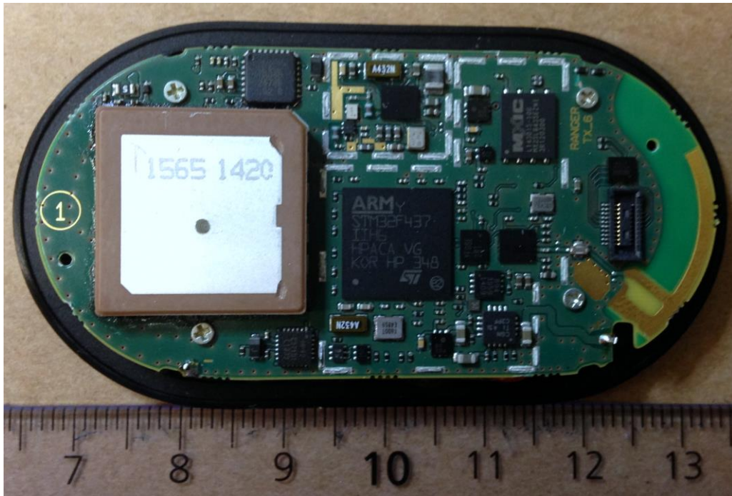
Figure 3. Electronics module without shields.
