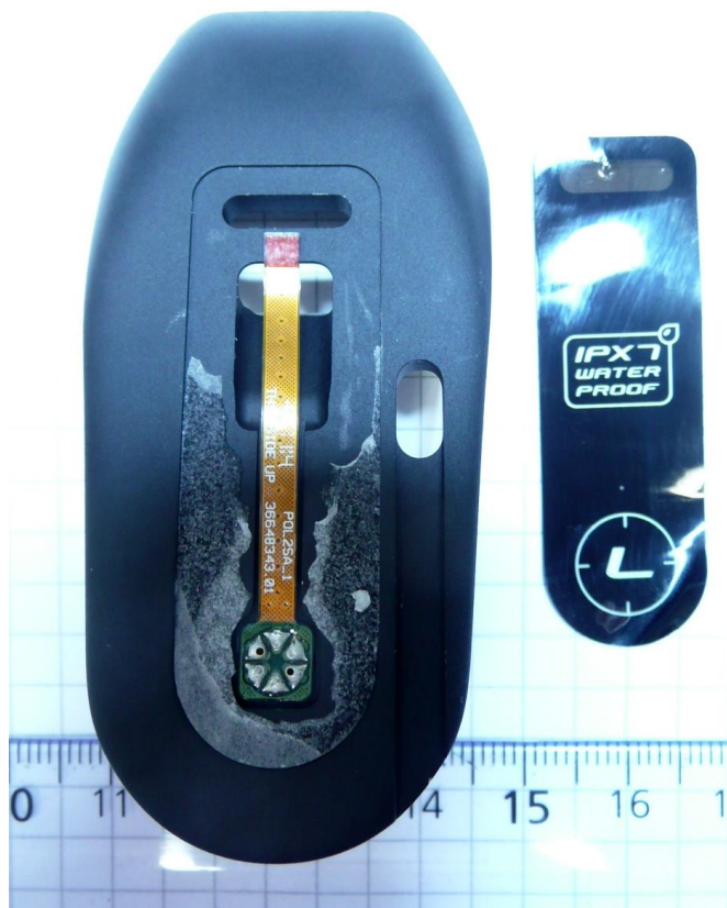
Figure 6. Back side, flex cable visible.
