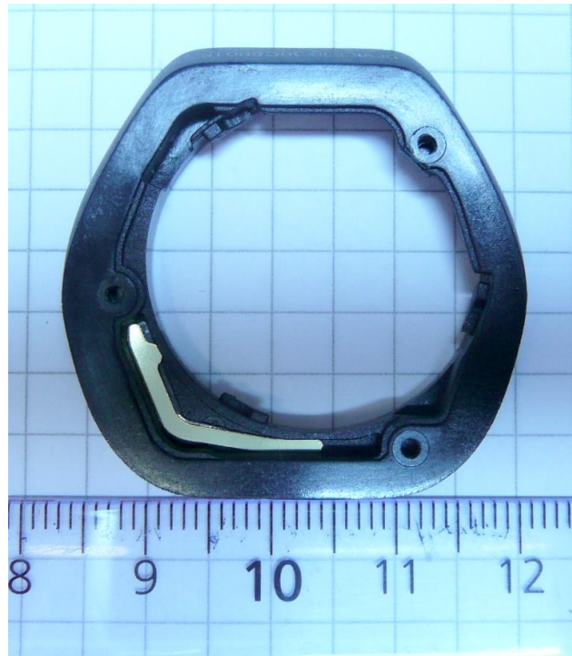
Figure 5. Antenna integrated into battery frame.
