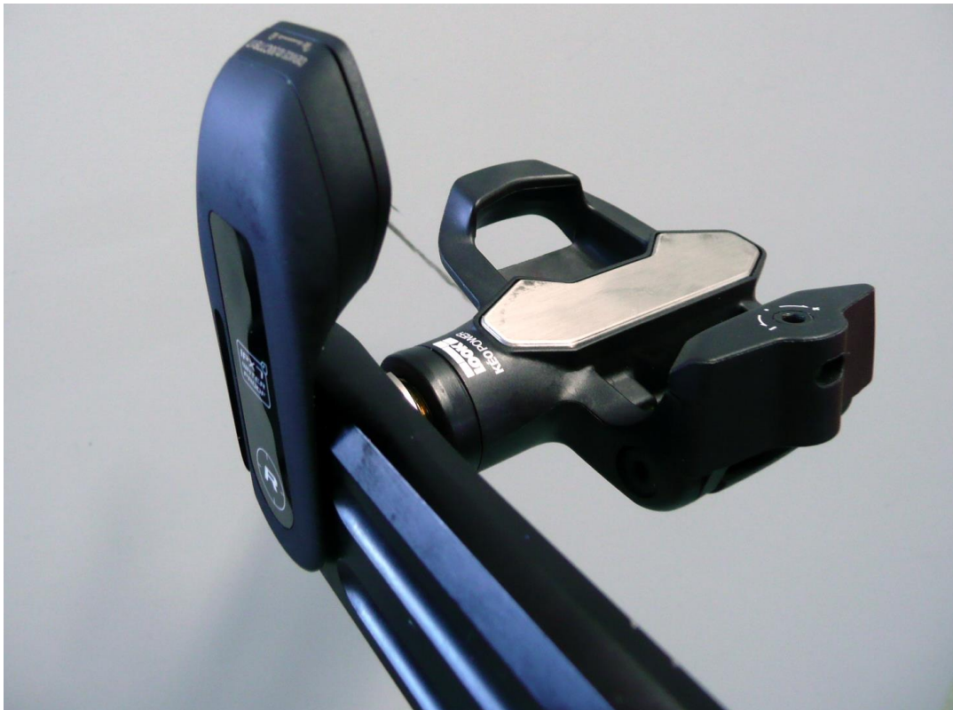
Figure 4. Module connected to a pedal and crank.
