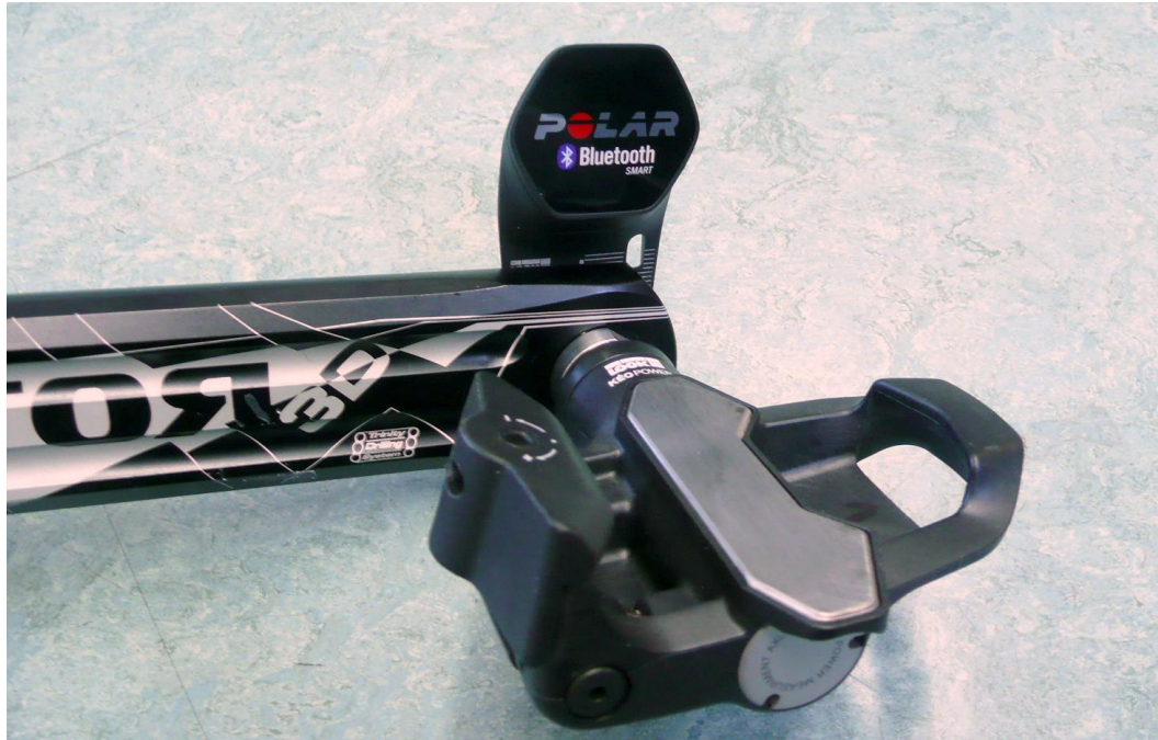
Figure 3. Module connected to a pedal and crank.
