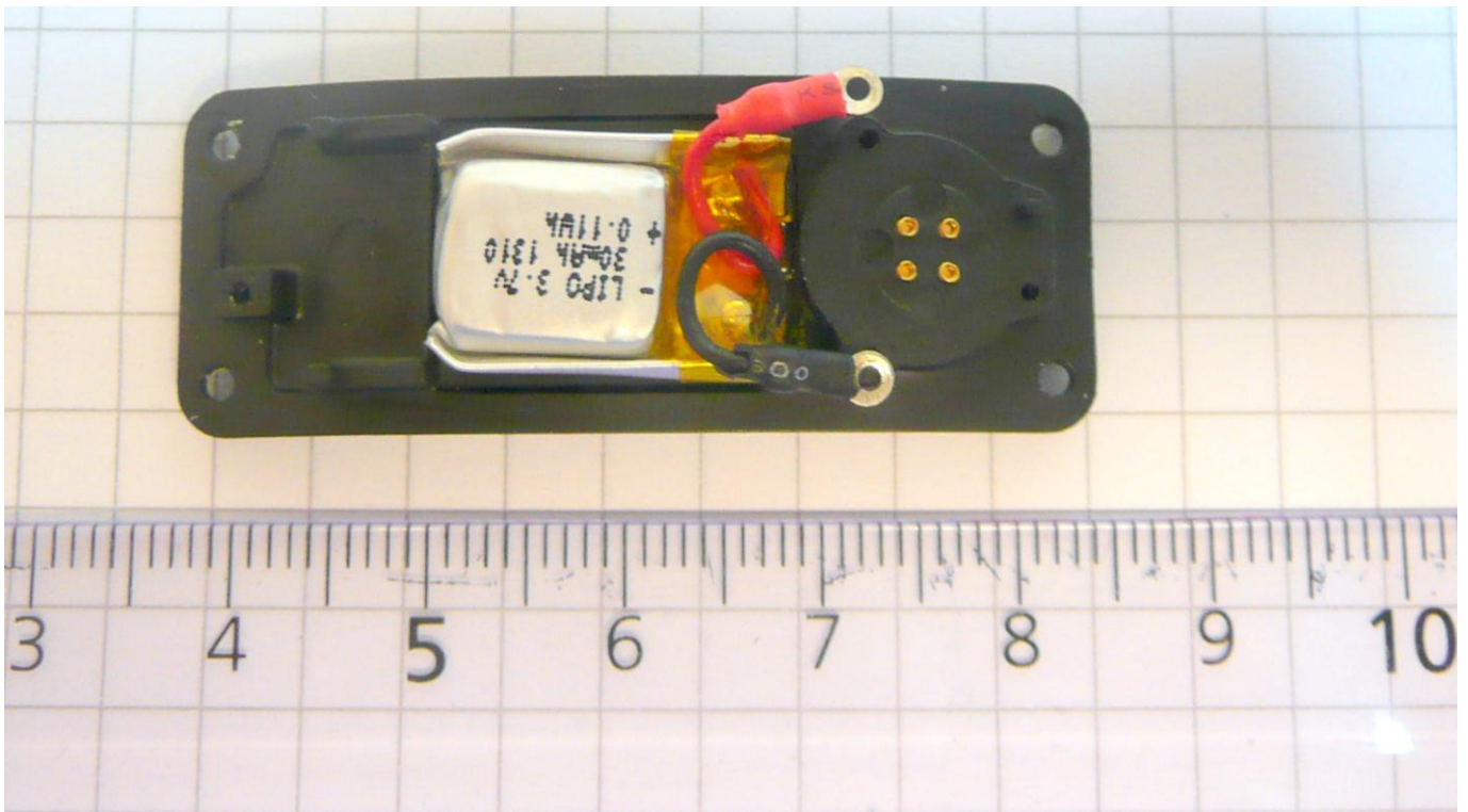
Figure 7. Battery on the back plate
