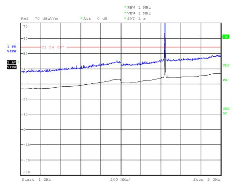
Note: The peak shown in the plot above the limit is the carrier frequency.
