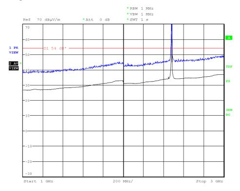
Note: The peak shown in the plot above the limit is the carrier frequency.
