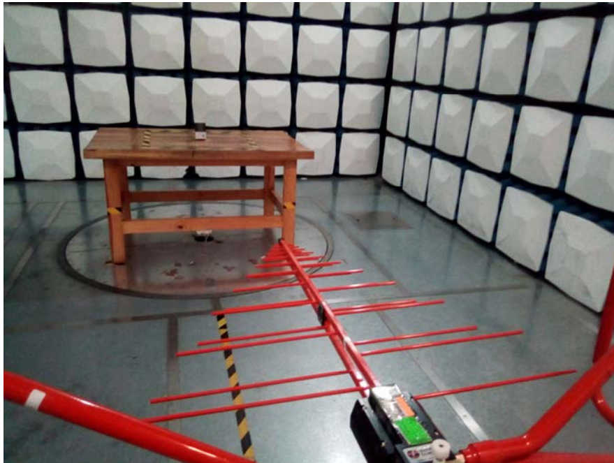
Radiated Emission Below 1GHz – Front View
