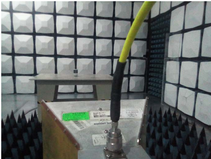
Radiated Emission Above 1GHz – Front View
