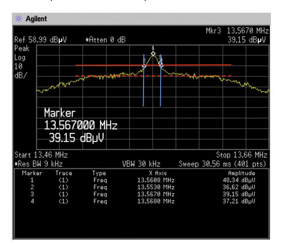
Point 1 amplitude =  $48.3 \text{ dB}\mu\text{V}$ Red dotted line amplitude =  $29.0 \text{ dB}\mu\text{V}$ Solid red line amplitude =  $39.2 \text{ dB}\mu\text{V}$
