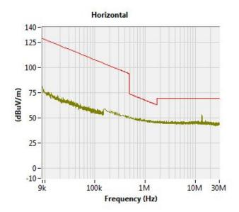
9kHz - 30MHz, Antenna: Magnetic Loop at 3m
