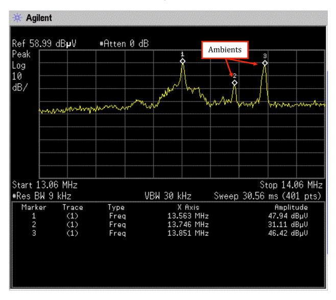
Note: Peaks 2 and 3 are ambient signals; i.e., not from the EUT. These signals were present with the EUT powered off.
