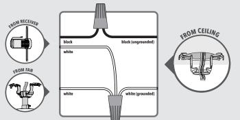
Turn the splices upward and push them carefully back through the hanger bracket into the outlet box. Spread the wires apart, with the grounded wires on one side of the outlet box and the ungrounded ires on the other side of the outlet box.
