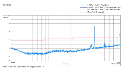
Note: Emission at 433.93 MHz was the carrier. Peak scan. Average Limit Line
