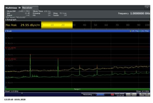
Note: Radiated spurious emissions measurements were performed from 30 MHz to 4.5 GHz.
