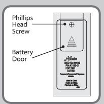
Installing or changing the battery -To access the battery compartment remove the small Phillips head screw that secures the battery door to the transmitter assembly. Replace with a CR2032 battery when necessary. The battery should be installed with the positive (+) side up.
