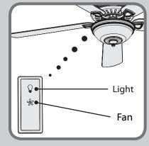
before the fan will operate. Within 3 minutes of restoring power to the fan, press both the Fan button and the Light button for at least 4 seconds. The remote is now paired to the fan's receiver. If using the transmitter with multiple fans, repeat this process for each fan.
