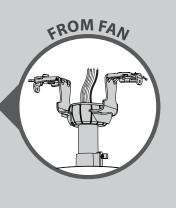
CONNECT WIRES FROM RECEIVER TO FAN -Using the blue wire connectors connect the white wire from the receiver (marked "common out") to the white wire from fan. Connect the black wire from the receiver (marked "fan out") to the black wire from the fan. Connect the blue wire from the receiver (marked "light out") to the blue wire (or possibly black with white stripe) from the fan.
