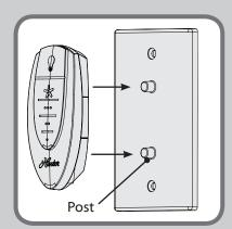
Your 3-Speed Remote comes with a wall plate that has two (2) posts on which to mount your transmitter when
