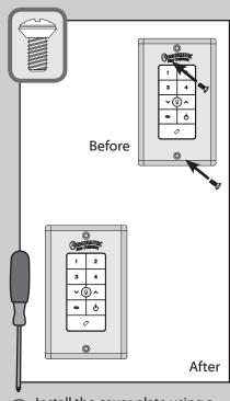
Install the cover plate using a Phillips Head screwdriver to secure the two cover plate screws.
