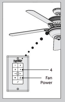
The fan must be paired before it will operate. Press the "4" button and the fan power button simultaneously for at least three seconds. The fan will turn at the lowest speed signifying that the remote pairing process is complete.
