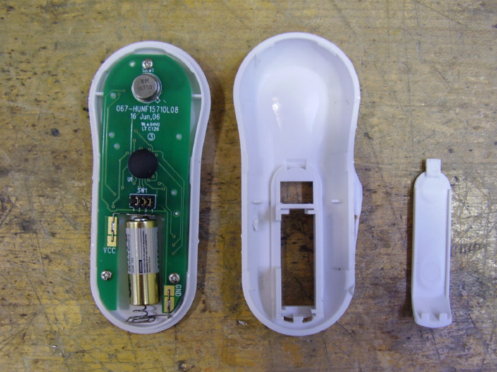
Model 27157 Transmitter – Circuit Board – SAW Resonator/IC side with case
