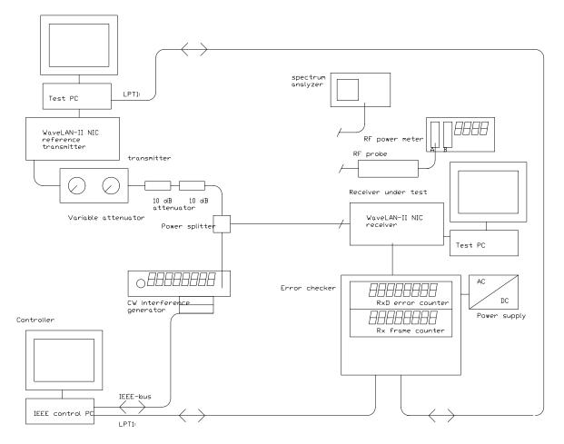
Figure 1, measurement test set-up.
