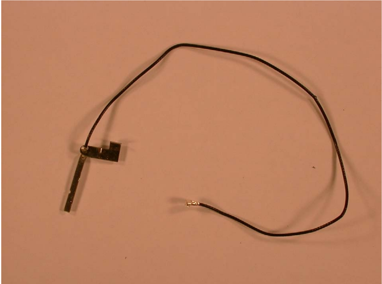
Photograph 13 – Antenna assembly of Latitude C600
