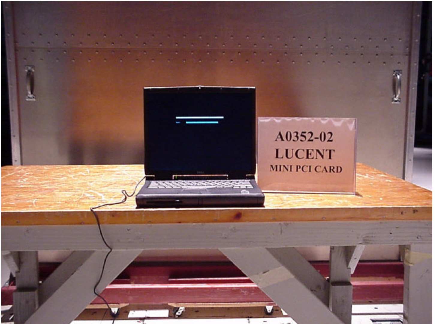
Photograph of Test Setup: Conducted Emissions 10/150/450 kHz - 30 MHz
