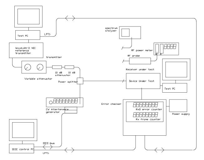
Figure 1, measurement test set-up.
