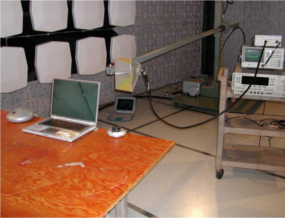
Figure 5.3: front picture of test configuration, for testing above 1 GHz.
