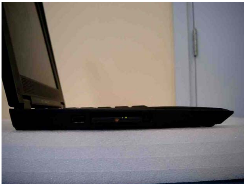
Figure 4: Side view. Offset Card to base = 13 mm
