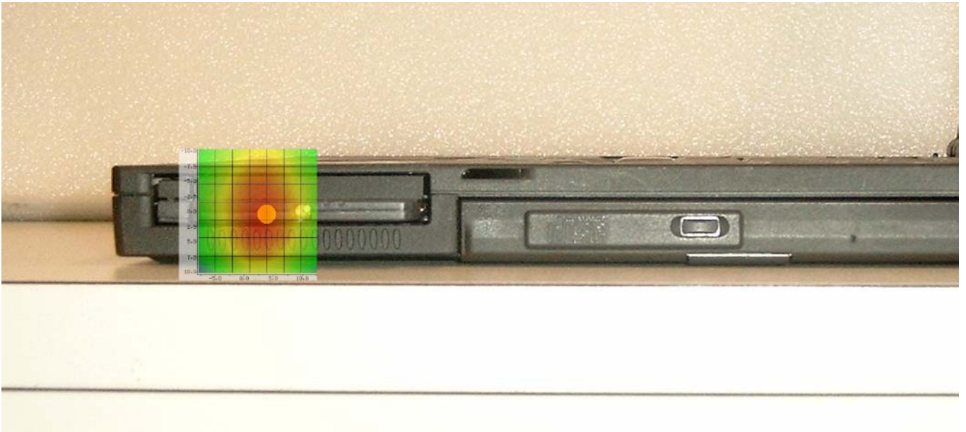
Photo 7 A 2d scan giving the field strength in the first scanned plane, overlaid on a bottom view photo of the laptop. Overlaid plot is that of the worst case perpendicular scan in channel 64
