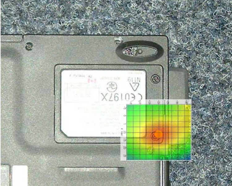
Photo 6: A 2d scan overlay giving the field strength in the first scanned plane, overlaid on a bottom side view photo of the laptop. 2d scan is that of the worst case lapheld value in channel 6.
