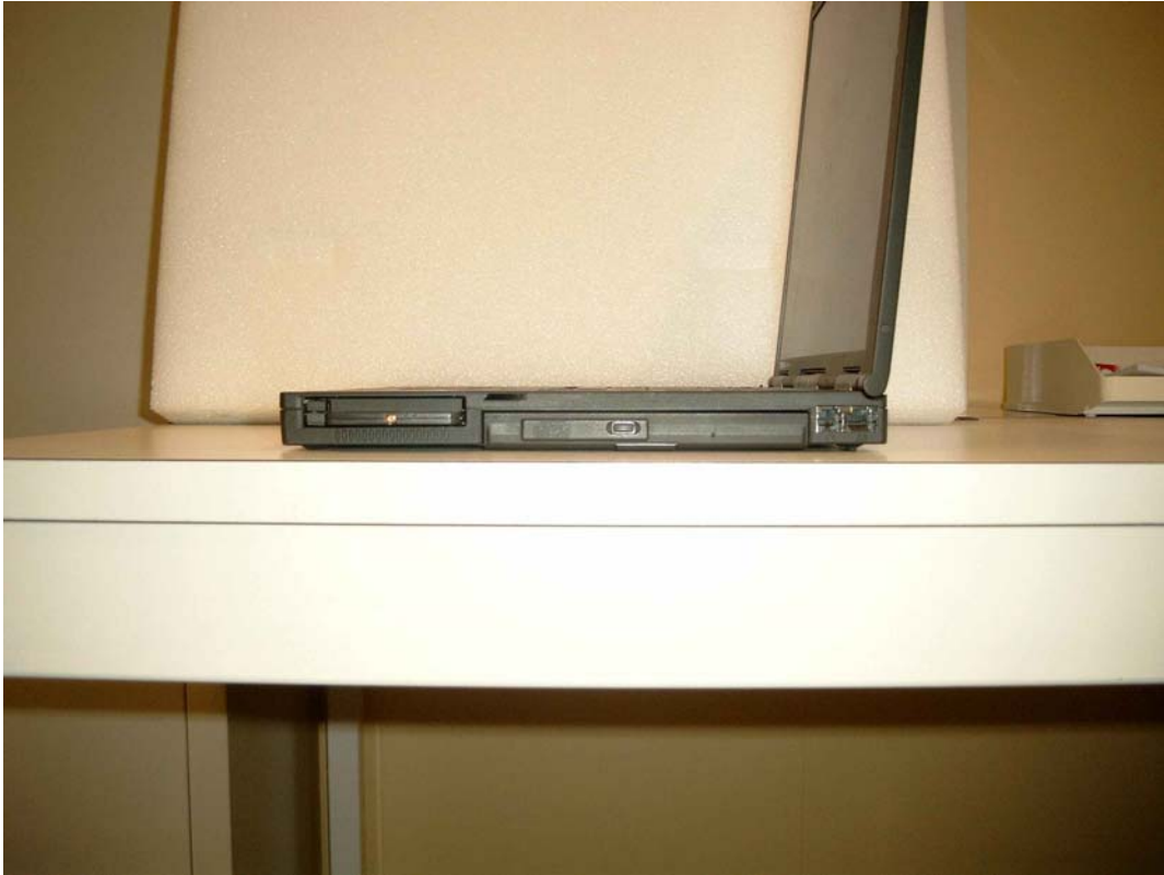
Figure 4 : Side view. Offset Card to base = 13 mm
