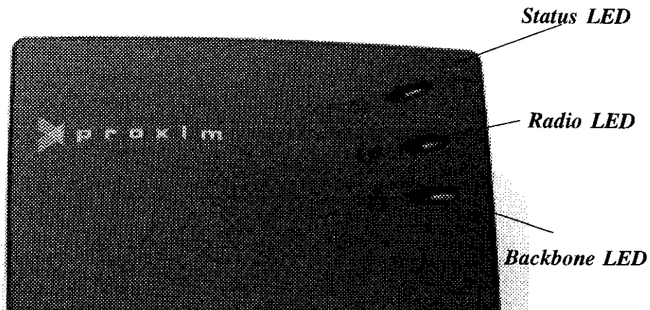
Figure 11 Front Panel LEDs
