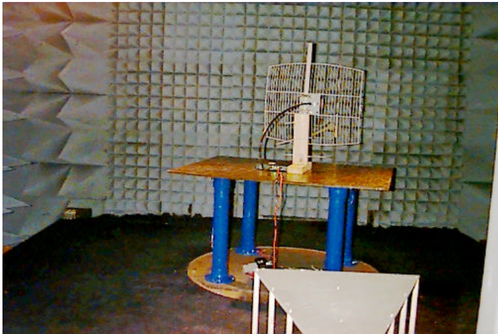
Parabolic Dish Antenna –Rear
