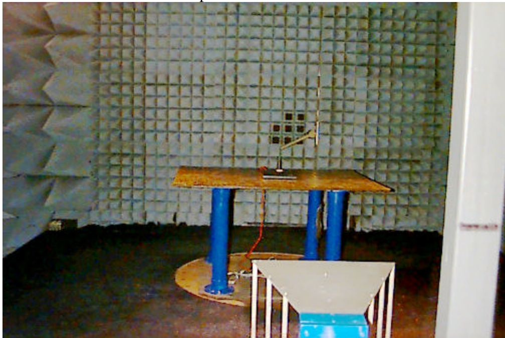
Dipole Antenna –Rear
