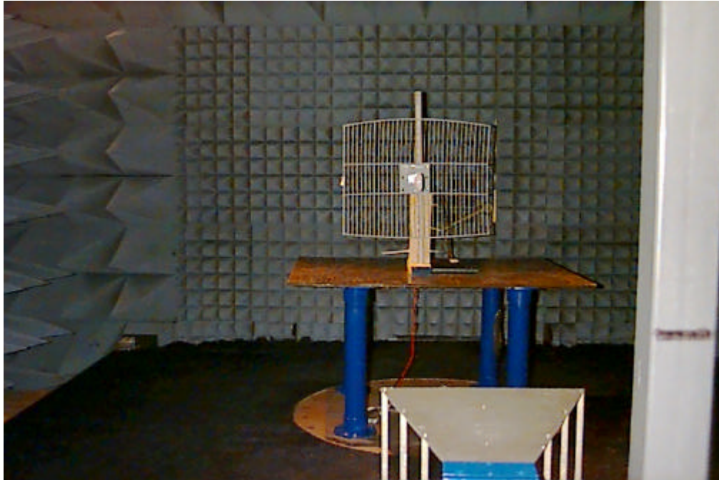
Parabolic Dish Antenna – Front
