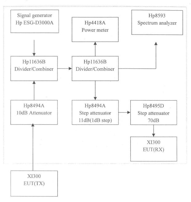
Processing gain test setup
