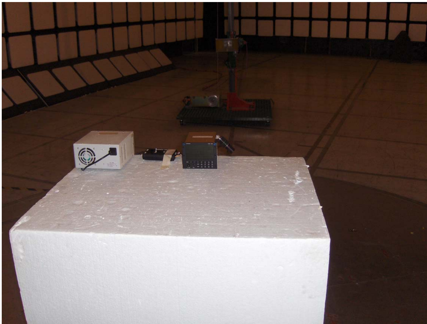
Plot #1: Radiated Emission Test Setup
