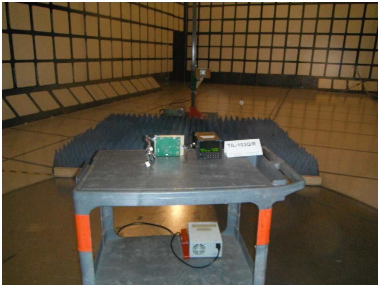
Radiated Emissions at 3 m, Above 1 GHz, Orthogonal Position 3
