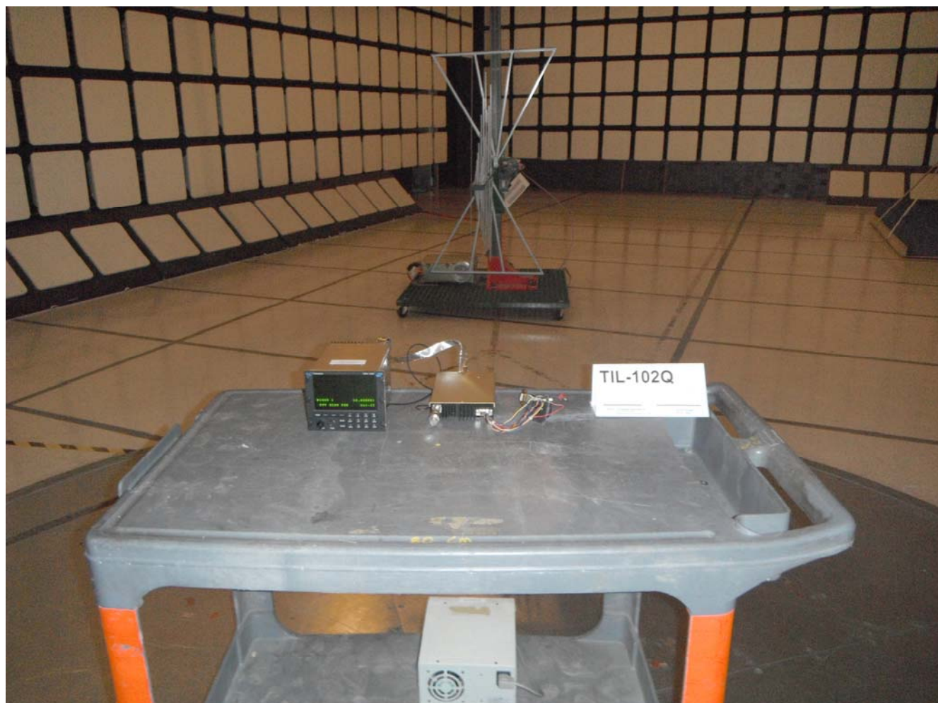
Radiated Emissions at 3 m, 30 - 1000 MHz Orthogonal Position 1
