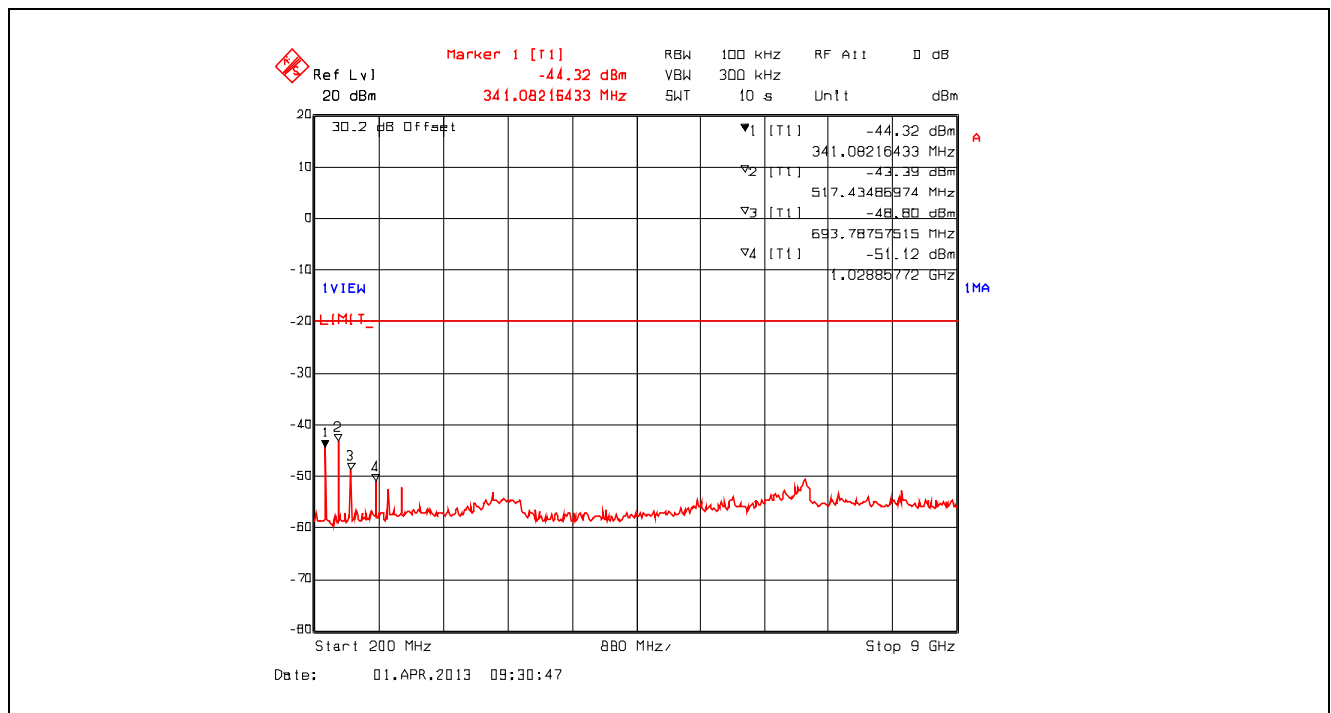
Plot 5.5.4.14. Conducted Transmitter Spurious Emissions, High Power, 173.3 MHz, 200 MHz - 9 GHz
