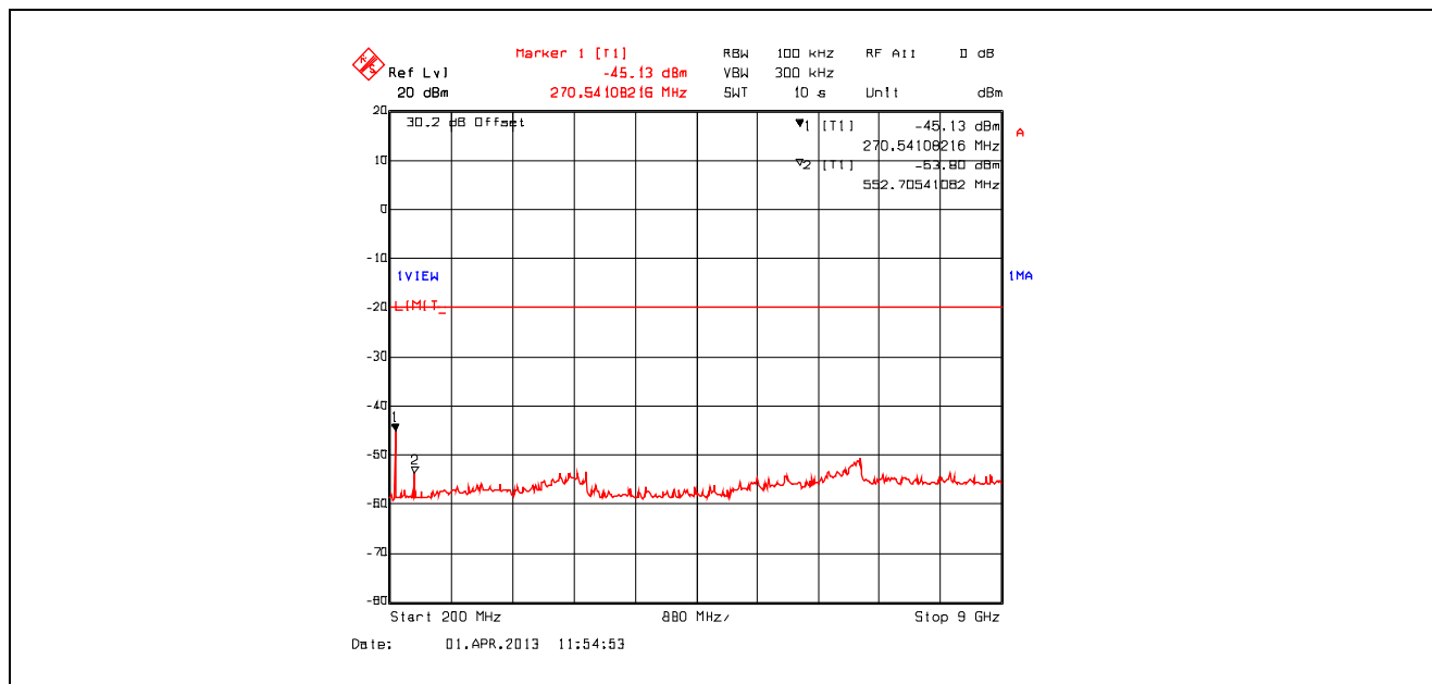
Plot 5.5.4.2. Conducted Transmitter Spurious Emissions, High Power, 138.1 MHz, 200 MHz -9 GHz
