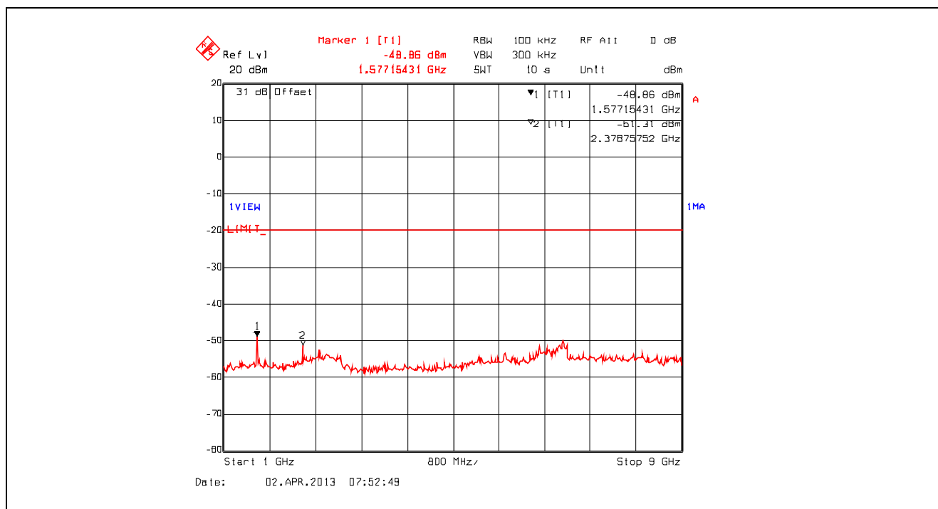
Plot 5.5.4.32. Conducted Transmitter Spurious Emissions, Low Power, 794.1 MHz, 1 GHz - 9 GHz
